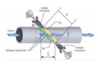
$$V = \frac{P^2}{2L} \frac{\left(t_{up}^{-} t_{dn}\right)}{t_{dn}^{\times} t_{up}}$$
