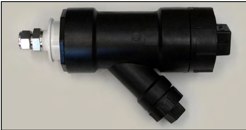
Figure C-6. Zero Flow calibration chamber — assembled
