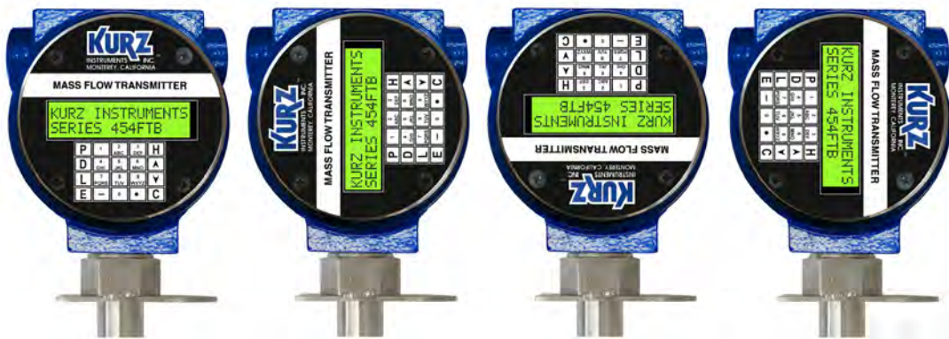
Figure 2-7. Display/keypad rotation (with cover removed)
