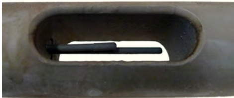
Example of Dirty Sensor
