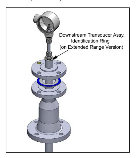
**6.** Line up the flange holes and bolt the packing gland to the isolation valve.
