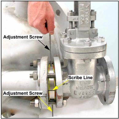
Figure 6: Adjusting the Wedge Position
