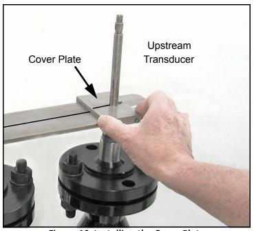
Figure 10: Installing the Cover Plate
