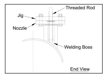
**4.** Align the nozzle scribe marks with the pipe scribe marks and tighten the assembly in place using the 1-in. washer and nut provided. If slight misalignment occurs between the nozzle scribe marks and pipe scribe marks, loosen the four bolts holding the jig and nozzle assembly, and rotate the nozzle for the best alignment. After the nozzle has been accurately aligned, retighten the four bolts.
