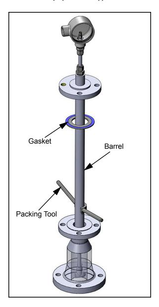
2. Check and make sure the isolation valves are securely installed with gaskets and hardware. Then, place a gasket on the face of each isolation valve (see either *Figure 14* below or *Figure 15 on page 48*).
