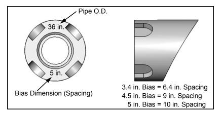
2. Check the spacing between the holes on the alignment plate, as shown below. The dimensions should correspond to the bias/spacing dimension on the welding boss.
