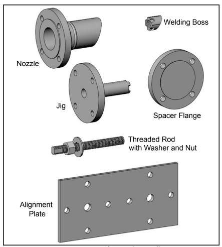
Figure 1: Components for Nozzle Installation Kit
