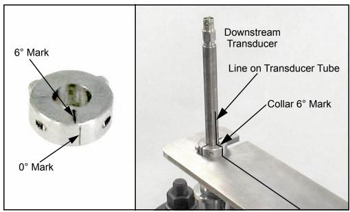
Figure 11: Installing the Locking Collar
