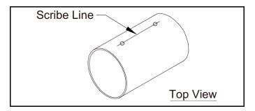
5. Along the new scribe line, mark off a length equal to your transducer spacing (10 in., 9 in. or 6.4 in.) and scribe two lines at least 10 in. in length and perpendicular to the scribe line on different sides of the scribe line.
