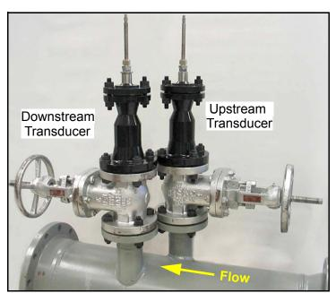
Figure 8: Extended Range Transducer Installation
