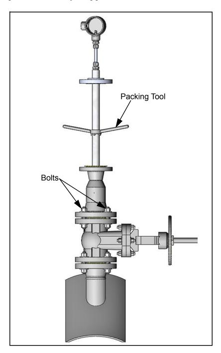
7. Using the packing tool, tighten the packing nut again so the nut is recessed.
