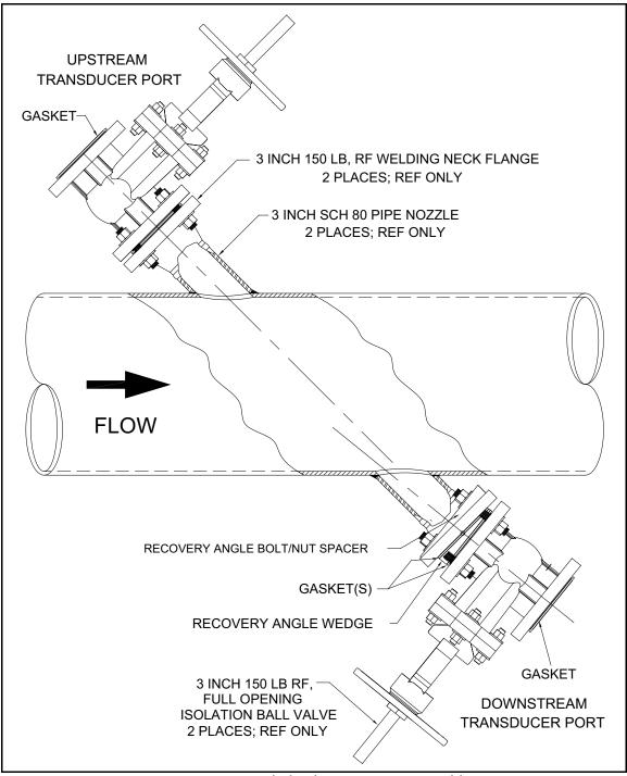
Figure 15: Extended Velocity Range Assembly
