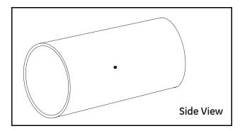
**4.** Spray this area with a marking dye product. Using a metal straight edge, scribe 6 in. long vertical and horizontal lines that intersect at the center punch mark.
