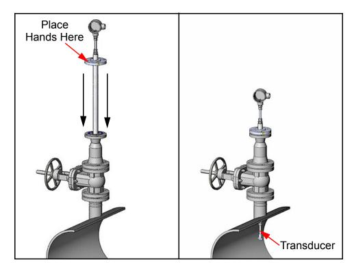
**4.** For this Bias 90 configuration, orient the alignment marks on each barrel flange so that they are facing each other. The alignment mark, which is marked with yellow paint, is scribed on the top and outside of the flange.
