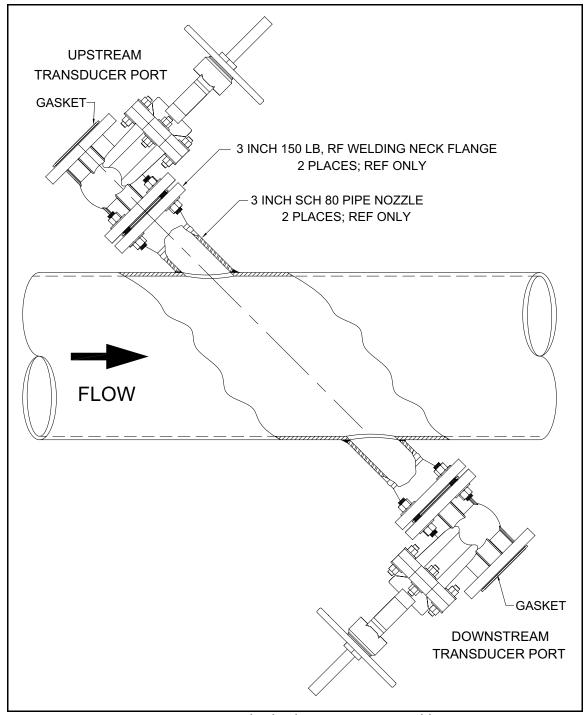
Figure 14: Standard Velocity Range Assembly
