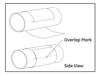
**5.** Remove the strip of film and fold it as shown below to determine the position which is diametrically opposite the overlap position when the film is reapplied to the pipe.
