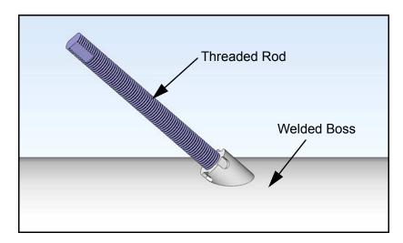
2. Slide the nozzle over the threaded rod, and align the contoured end of the nozzle so that it matches the pipe arc. Then slide the jig over the threaded rod and fit the jig into the welding boss.
