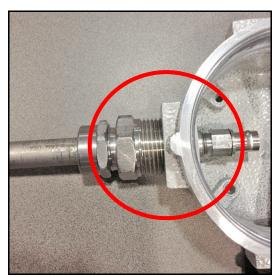
Figure 16: Torquing the NPT Reducer
