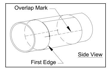
**8.** The new location of the center of the second nozzle is now identified as the intersection of the fold line and the second edge of the strip of film. Center punch this location prior to removing the strip of film.
