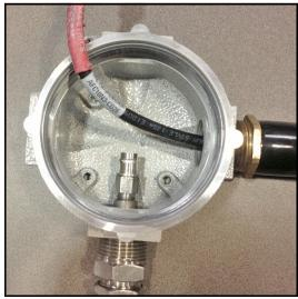
Figure 18: Assembled Transducer and Cable Gland
