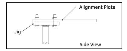
2. Screw the threaded rod into the second boss. Then, insert the bolt/boss assembly into the jig key cut grooves and secure it with a washer and nut on top.
