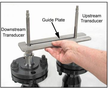
Figure 9: Installing the Guide Plate
