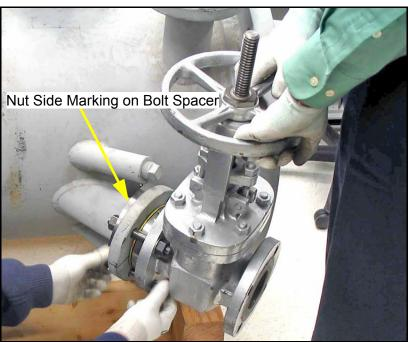
Figure 5: Mounting the Isolation Valve
