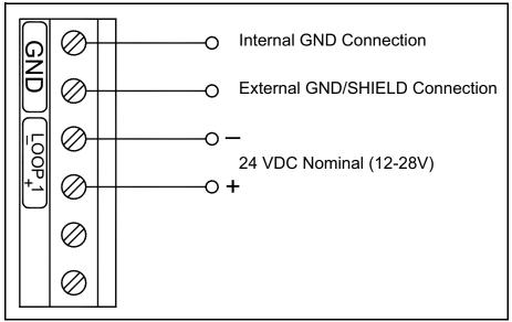
**Figure 13: Electrical Connections**
