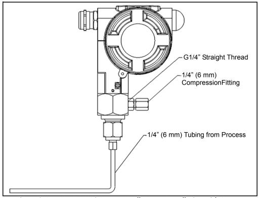
Figure 8: DewPro MMY 30 Remote Wall-Mount Installation with Bypass
