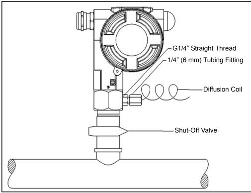
Figure 6: DewPro MMY30 Installation at Inlet Orifice
