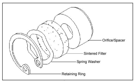
Figure 16: Filter Components
