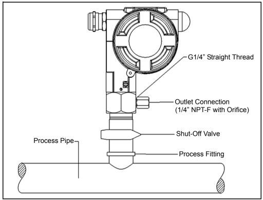
Figure 5: DewPro MMY30 Installation at Outlet Orifice
