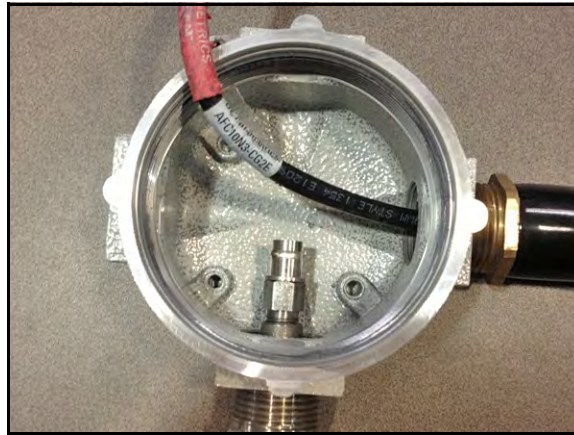
Figure 10: Assembled Transducer and Cable Gland
