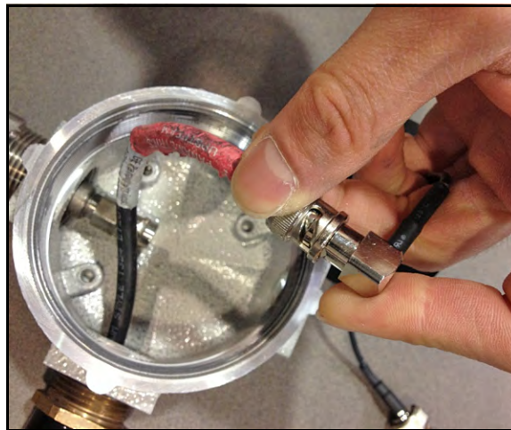
Figure 11: Connecting BNC Plug to Cable
