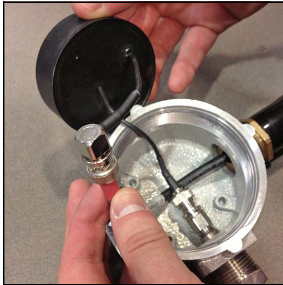
Figure 12: Female Plug to Male BNC Head
