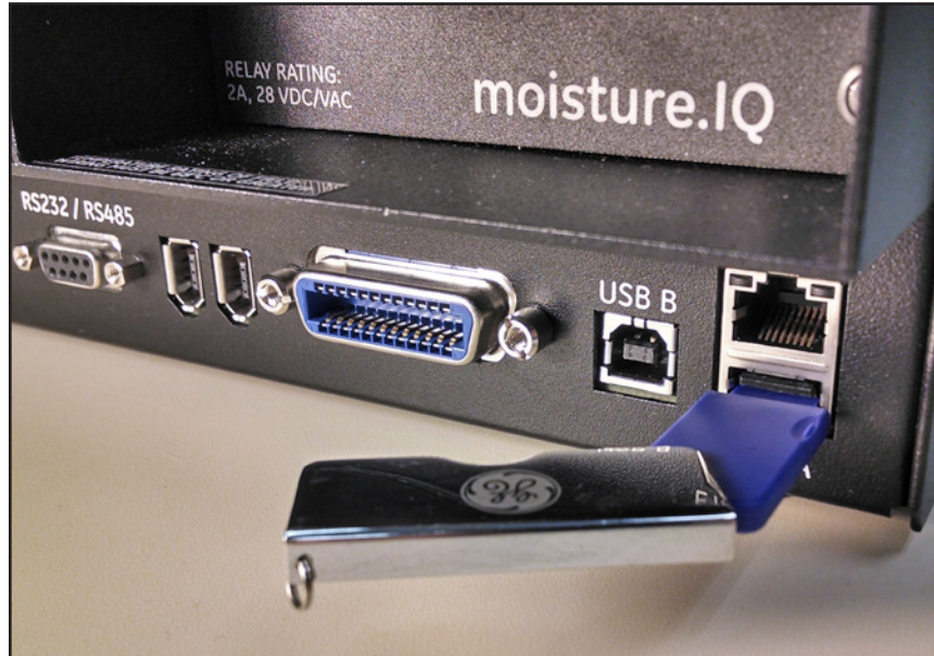
Figure 84: USB Flash Drive Plugged into Rear of Chassis
