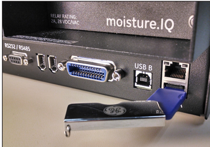
Figure 91: USB Flash Drive Plugged into Rear of Chassis
